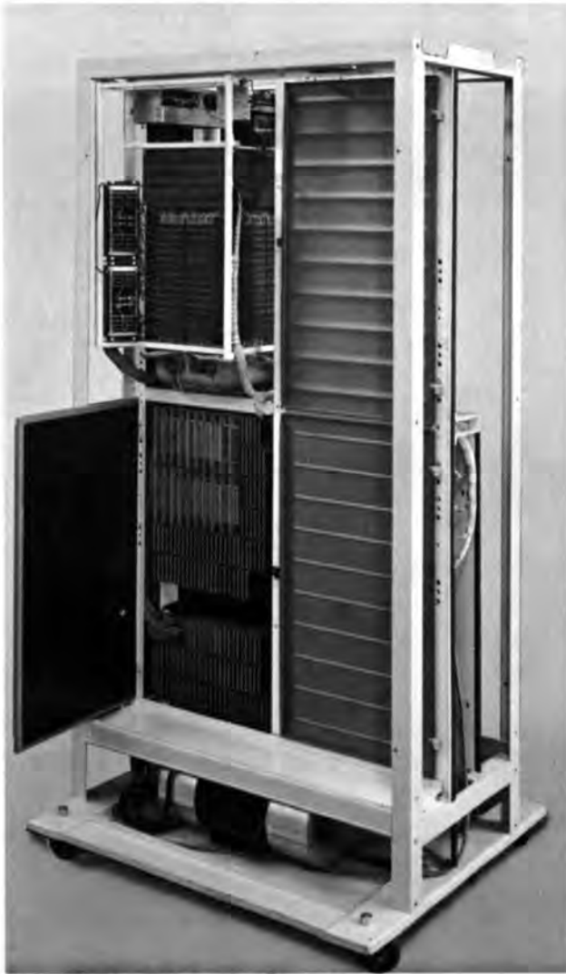
Figure 16. Fixed Gate Frame Assembly Rear
