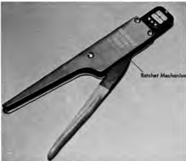
Figure 38. M8ND Tool with Die-Set Installed
