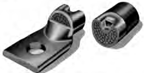
Figure 36. Crimped Connection, Cross Section
